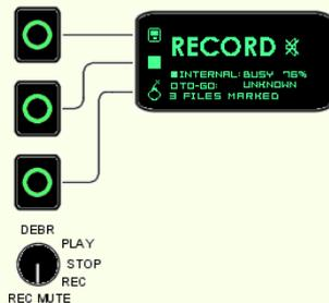
Allows the operator to record video without audio.
